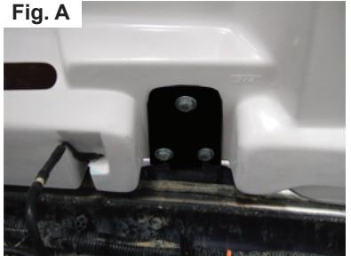
**STEP 2:** Bolt the hood to the top of the hinges with the supplied 3/4 inch bolts and washers **as shown in fig.A.**
