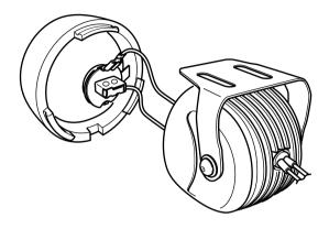
Snap front lens unit off from housing. Be careful not to pull too hard and damage wires.
