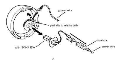
When service is complete snap lens unit back onto housing being careful not to pinch any wires.
