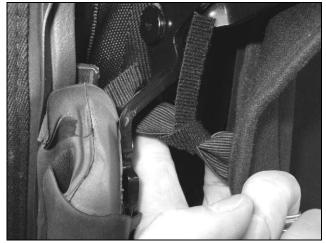
C) Wrap the top leg around frame and secure Velcro Strap to the frame with the bottom leg of the Velcro Strap, as shown.
