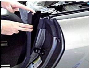
C) Use a Door Trim Tool (Fork Tool) to dislodge the pushpin retainer at the rear edge of the Trim Panel approximately 4" down from the top, pry Trim Panel toward the outside of car to release retainer.
