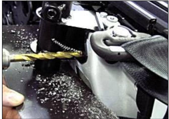
**Note:** It is very important that you protect the seat belt and the shoulder strap retractor from the cutting debris that is created during the drilling process. We recommend using a magnet or drop cloth to catch the debris.
