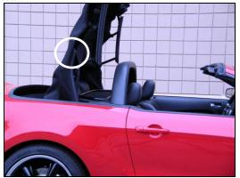
B) Use the 6" Velcro straps (CDC # 950009) to draw the elastic band tight. Cross the Velcro Strap around the elastic band. Route the top leg of the Velcro Strap **behind** the frame. **IT IS IMPORTANT THAT THE TOP LEG GO UNDER THE FRAME!**
