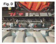
**Step 4:** On the 6.1L motor you need to remove the Hemi fuel rail covers. On the 5.7L motor you will need to remove the engine cover. Pull up on cover and it will release the clips **as shown in fig.D.** Remove the vent hose from the car completly and install the supplied air breather to the intake manifold where the vent tube used to be **as shown in fig.E.**
