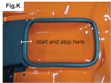
**STEP 8:** Install the rubber seal to the underside of the hood **as shown in fig.K.**
