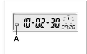
If the batteries are removed or fail, the keypad memory will NOT be erased and the active programmed code will still work once power has been restored.
